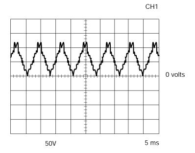
This is the typical DC output voltage generated from a properly operating machine. Note that each vertical division represents 50 volts and that each horizontal division represents 5 milliseconds in time.
